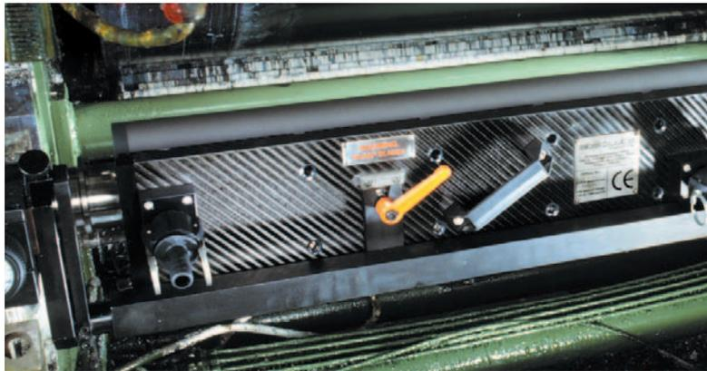
**I-Max is an ink maximisation system, consisting of two elements, an integral wiper shuttle which resides permanently in the ink cavity, and an external linear drive unit.**
