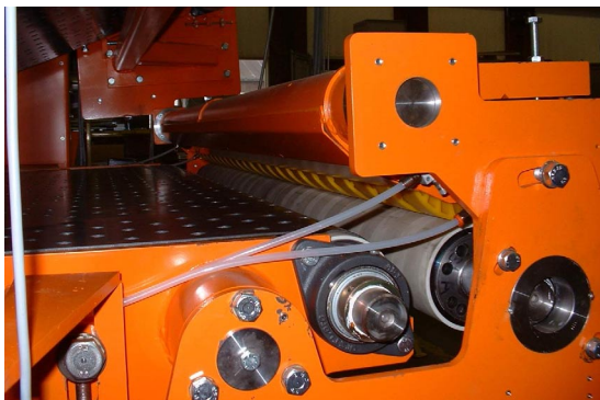
Acceleration roller with end of belt conveyor
