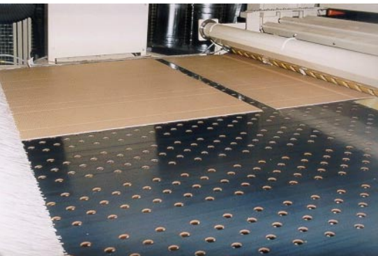
Full width conveyor belt with 2 vacuum sections
